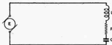
Figure 27. Schematic of a series-resonant circuit containing resistance.
